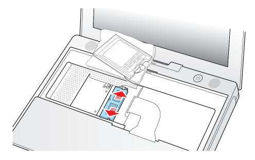
3. Install the replacement memory card by lining up the notch in the memory card with the small tab in the memory slot. Hold the card at a 30-degree angle, then push the card into the slot until it is firmly seated.
