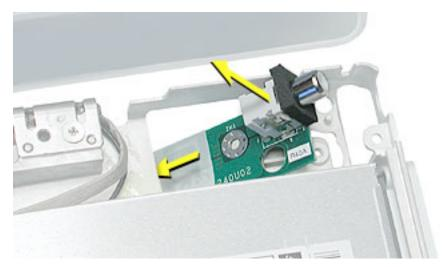
3. Disconnect the flat power cable from the connector on the logic board.
