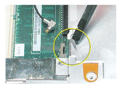
4. Before lifting up the top shield, note that the shield fits over posts on the computer frame.
