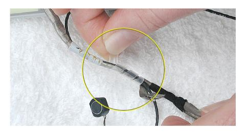
6. Remove the microphone cable from the assembly.
