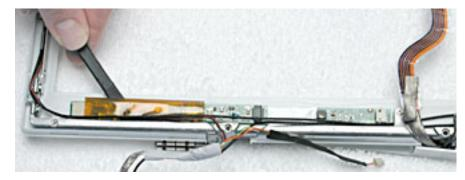
**Replacement Note:** The inverter board is held to the bezel assembly with double-sided tape on each end of the board. Use new double-sided tape when installing the replacement inverter board.
