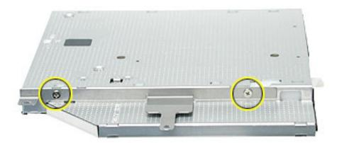
14. Install the replacement optical drive, and reassemble and test the computer.
