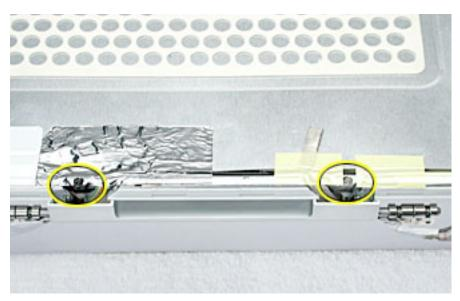
10. Loosen the remaining tape that secures the shield to the assembly. Remove the shield.
