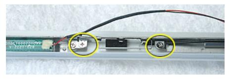
10. Tilt up the antenna receptor to remove it from the left side of the bezel assembly.
