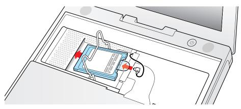
Use the wire holder to secure the AirPort Card in place by inserting its prongs into the slots in the RAM shield.
