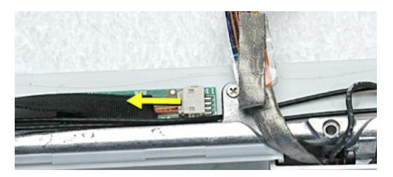
6. Remove the reed switch cable assembly.
