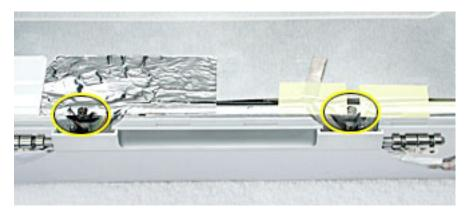
6. Tilt up the display assembly and pull straight down on the display clutch cover.
