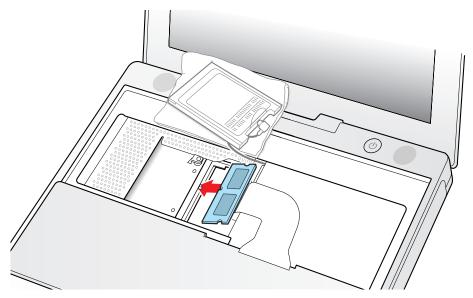
4. Gently push the top of the card down until the brackets snap onto both sides of the memory card to lock it into place.
