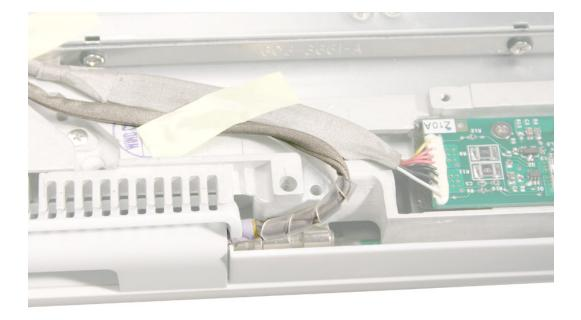
7. **Important:** Create enough slack in the cable near the connector to relieve tension on the cable. Secure the connector and cable with a strip of Kapton tape, as shown.
