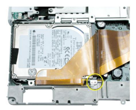
3. Warning: If the flex cable connector is pulled up unevenly, some connector pins could become bent and damaged.
