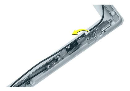
9. On the left side of the bezel, remove the two 3-mm long Phillips screws at the antenna receptor.
