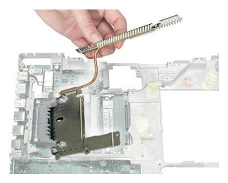
7. Turn over the heat spreader and notice the placement of the thermal pad on the other side. If replacing the heat spreader, make sure it has the thermal pad.
