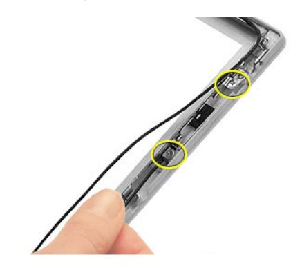
8. Tilt up the antenna receptor to remove it from the bezel assembly.
