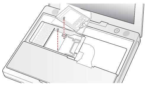
10. Lift the RAM shield out of the computer. Carefully pulling up on the wire holder may help to remove the shield.
