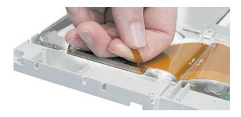
4. Lift up the fabric tape to release the microphone cable.
